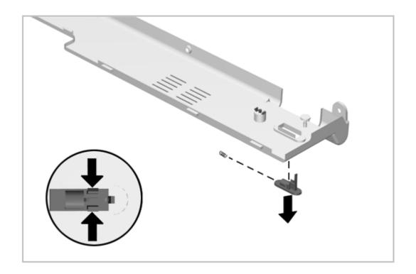
Figure 5-24. Removing the Power Switch Actuator
